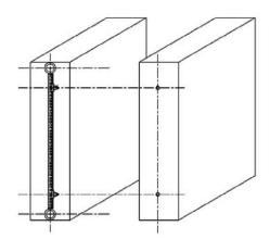
Scatterguard mounting diagram #1 Vertical & Horizontal Center Lines must be parallel for longest life. Step #2 To install ScatterGuard out of the box and without change to the assembled items see diagram 2. Care should be taken to locate magnets as specified in step 1 above.
