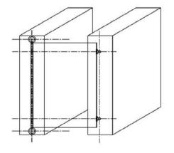
Scatterguard mounting diagram #2 Vertical & Horizontal Center Lines must be parallel for longest life.
